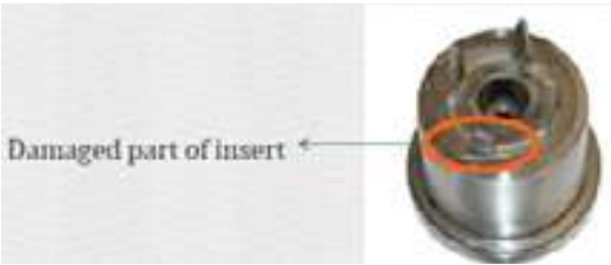
Figure 9 – ADDITIVE MANUFACTURING FOR REPAIRING DAMAGED INSERTS
