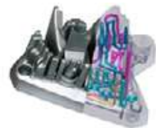
Figure 8 – 3 D PRINTING FOR CONFORMAL COOLING
