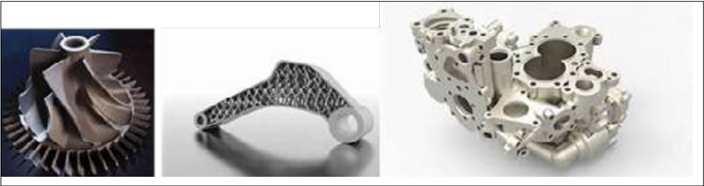
Figure 10 – EXAMPLES OF COMPONENTS MADE FROM DMLS PROCESS
