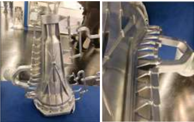
Figure 6 – GATING DESIGN FOR STRUCTURAL CASTINGS
